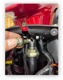
**13mm**. Turn the handlebars to to gain access to the nut side.
