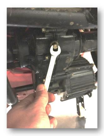
It is recommended to change the transaxle oil between from one to three years. Unlike a gasoline engine, the motor does not require a specific amount of oil to operate properly. It is strictly the lubrication method to avoid overheating in the differential assembly. There is a drain and fill bolt on the top and bottom of the motor. Drain old oil, replace fill bolt, and use 10W-30 motor oil to refill the transaxle, with approximately ½ quart.
