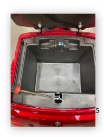
You're going to want to remove both wires going to the circuit breaker before removing the storage box.
