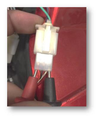
To test that the controller is emitting the proper voltage to the motor, connect your multimeter to any color combination on the motor phase wires where they connect at the yellow junction box. Set your meter at DC 50 or higher, and test under load (with the scooter power turned on, while pulling the throttle). The voltage should start at 0 and increase between 2.5-3.6 volts while under full load (holding the throttle pulled at the way).
