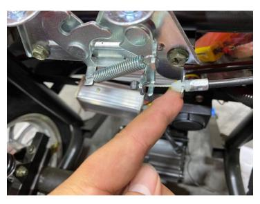
Remove the cable that goes to the truck lock. You're going to want to pull up in the meal/plastic part and remove the end of the cable.
