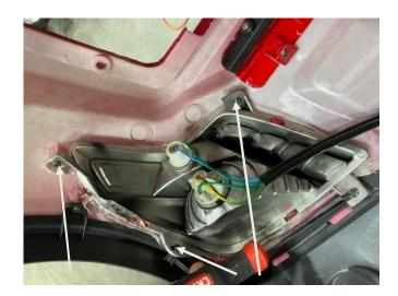
Remove all screw that attach the bumper to the body shroud on the inside. Keep in mind that there are going to be screws that go along the inside of the bumper.
