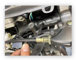
adjuster with securing washer to the point where the adjuster and washers cut outs match up with the cut out for the brake handle.
