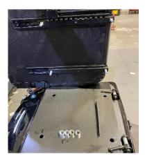
Remove all 4 bolts using a **13mm** socket with a rachet. Be careful as there are 4 spacers as well that will be.
