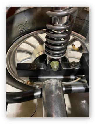
Once the rear wheels are removed, the next step is to remove the four 14mm axle to swing arm bolts. These bolts secure the transaxle assembly to the swing arms.
