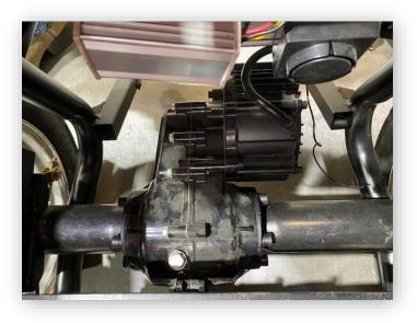
Going internal with the motor to determine if the differential, transfer case, motor hall sensors, or other internal components is the issue is not recommended for field service technicians. Typically, the labor costs for disassembling, testing, and reassembling will exceed the cost for a replacement motor. If the control unit is emitting the proper power to the motor under load, the brake sensor is not activated, and the rheostat is unplugged, and the motor is not engaging,
