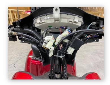
**Throttle Replacement** –To replace the throttle, start by removing the headset shroud. Once removed, separate the original throttle's electrical connector, and loosen (but do not remove) the 3 MM set screw for the original throttle. Disconnect both connectors and your job is complete.
