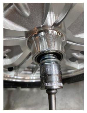
A jack or stand will be needed to remove the front tire. The front wheel is secured by the front axle bolt. On the wheel nuts there will be covers that need to just be popped off. The size you're going to need is going to be a 19mm socket to take this off.
