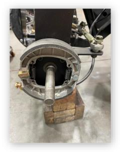
The brake pads are held onto the axle's brake pad catch, and to the actuating brake tension arm with spring tension. Pull the two sides of the brake pads away from each other to remove, and duplicate the reinstall the new pads
